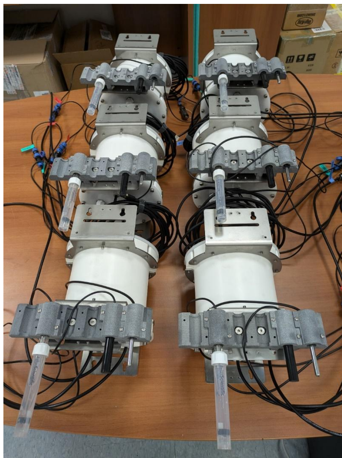
Figure 12. MDM CIRCE Units assembled to be used as RHE-MEDIation fixed nodes.
